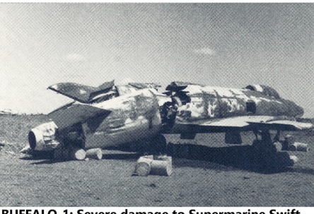
BUFFALO-1: Severe damage to Supermarine Swift
